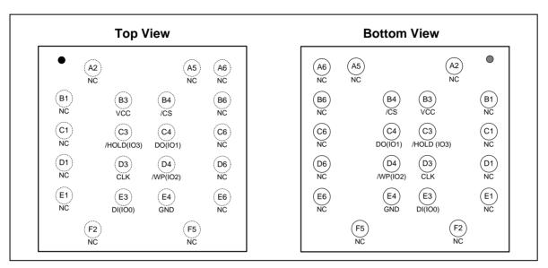
Figure 1e. W25Q128JW Ball Assignments, 21-ball WLCSP (Package Code Y)
