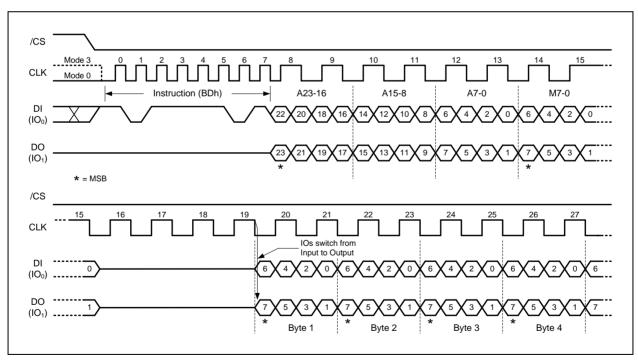
Figure 23a. DTR Fast Read Dual I/O (Initial instruction or previous M5-4≠10, SPI Mode only)
