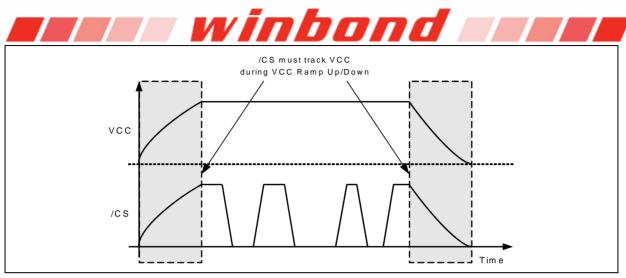
Figure 58b. Power-up, Power-Down Requirement
