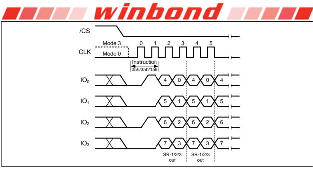
Figure 8b. Read Status Register Instruction (QPI Mode)
