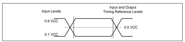
Figure 59. AC Measurement I/O Waveform
