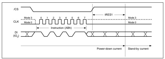
Figure 38a. Release Power-down Instruction (SPI Mode)
