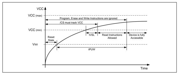
Figure 58a. Power-up Timing and Voltage Levels
