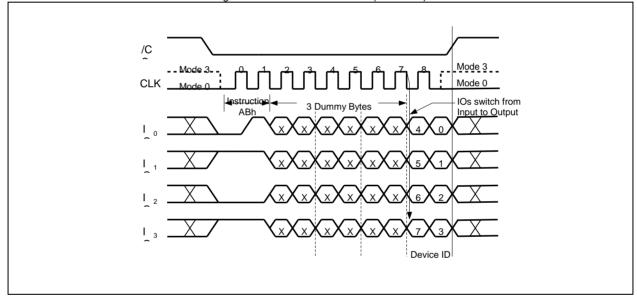
Figure 38d. Device ID Instruction (QPI Mode)
