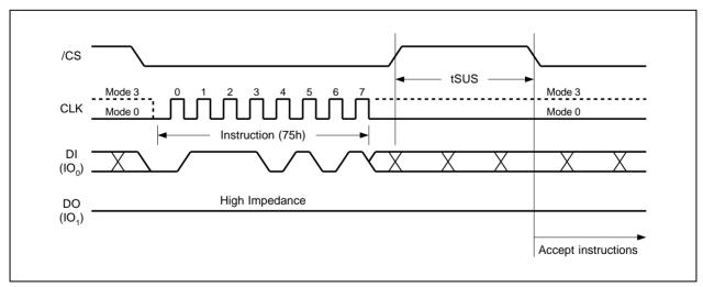
Figure 35a. Erase/Program Suspend Instruction (SPI Mode)
