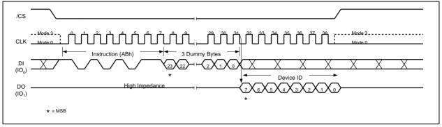
Figure 38c. Device ID Instruction (SPI Mode)
