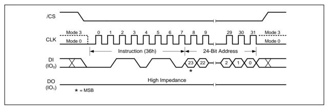
Figure 53a. Individual Block/Sector Lock Instruction (SPI Mode)
