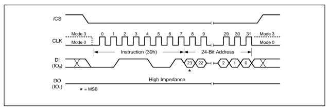
Figure 54a. Individual Block Unlock Instruction (SPI Mode)
