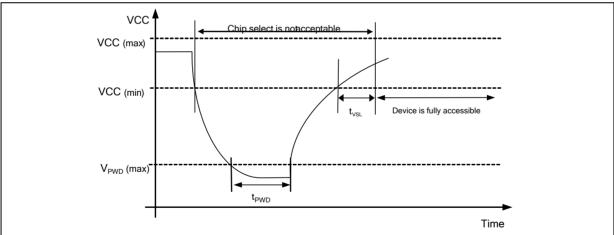
Figure 58c. Power Cycle Requirement
