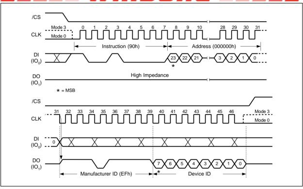
Figure 39. Read Manufacturer / Device ID Instruction (SPI Mode)
